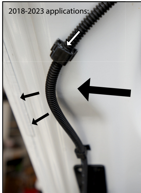
Gas spring housing attaches to hood
